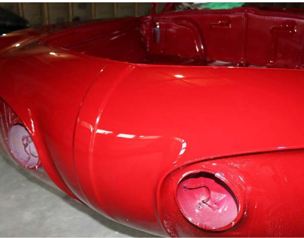
The body was media-blasted in mid-2013 and the finishing work was done by the end of 2013 (above). Since there were already three restored T34s in his area that were Sea Blue Scott decided to return it to its original solid Cherry Red.
