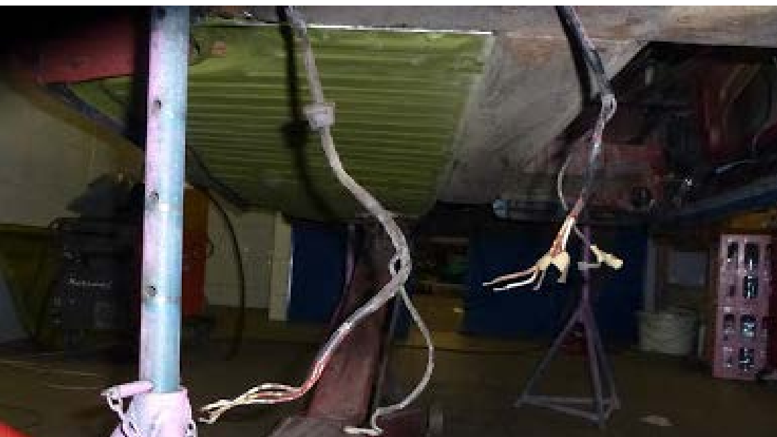
Below: When aligned, the new Gerson panels were welded into place.
