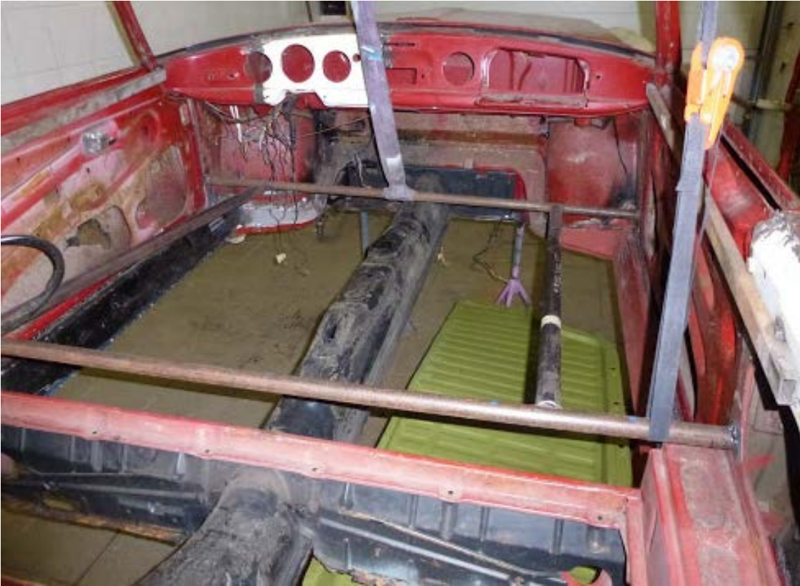
Above: To facilitate the alignment of the body mounting holes with the floorpan holes, Michael had the body mated onto the chassis again.
