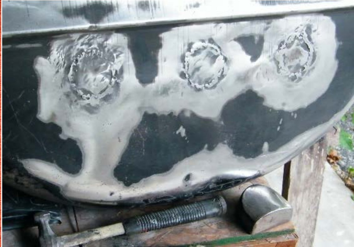
Old-school metal craftsmanship is the only way to fix the spare tire well.
