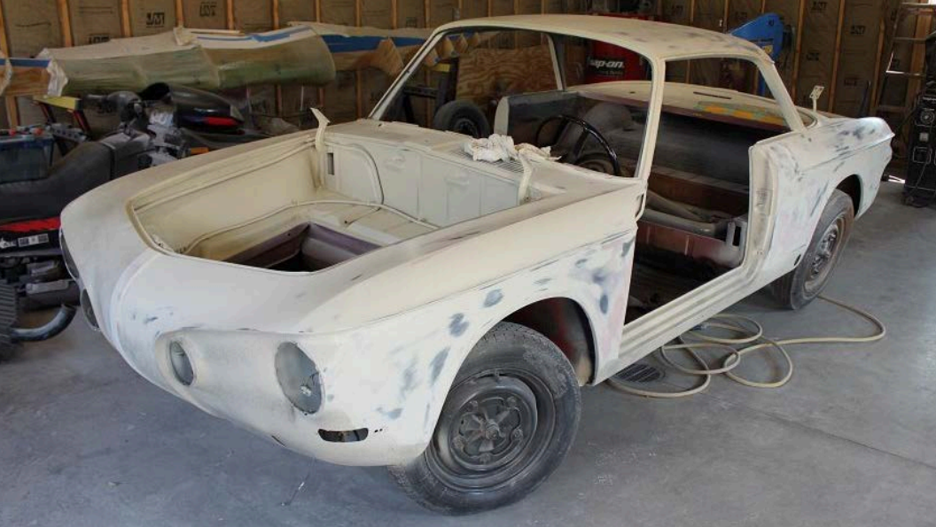
The body was media-blasted in mid-2013 and the finishing work was done by the end of 2013 (above). Since there were already three restored T34s in his area that were Sea Blue Scott decided to return it to its original solid Cherry Red.
