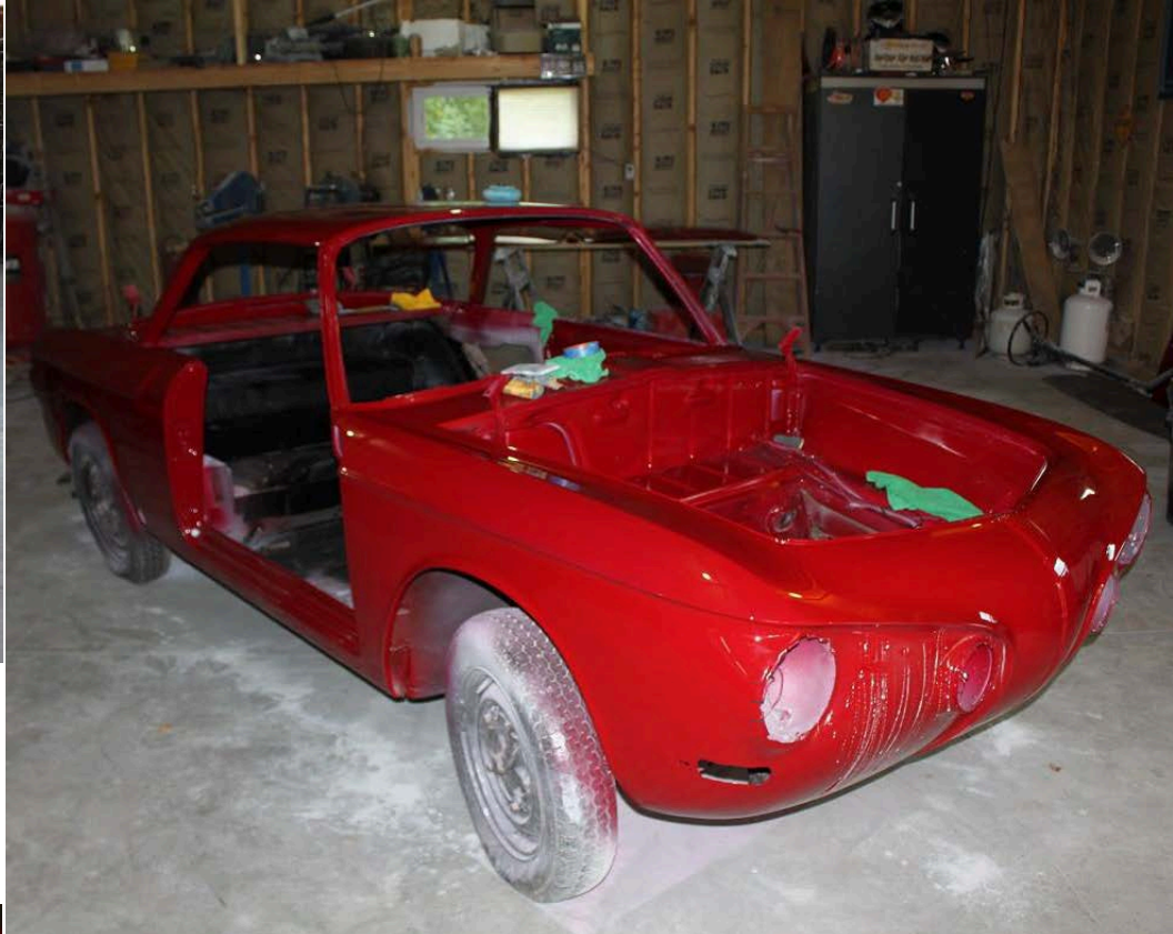
The body was media-blasted in mid-2013 and the finishing work was done by the end of 2013 (above). Since there were already three restored T34s in his area that were Sea Blue Scott decided to return it to its original solid Cherry Red.
