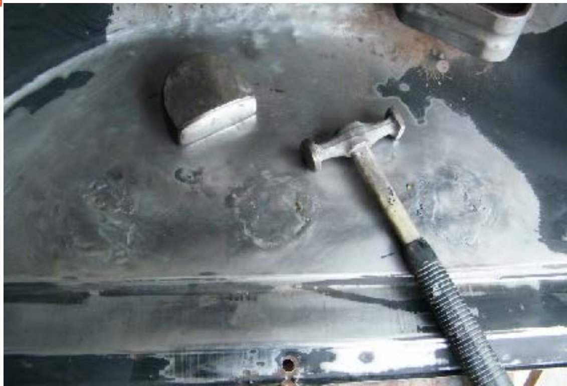
Old-school metal craftsmanship is the only way to fix the spare tire well.
