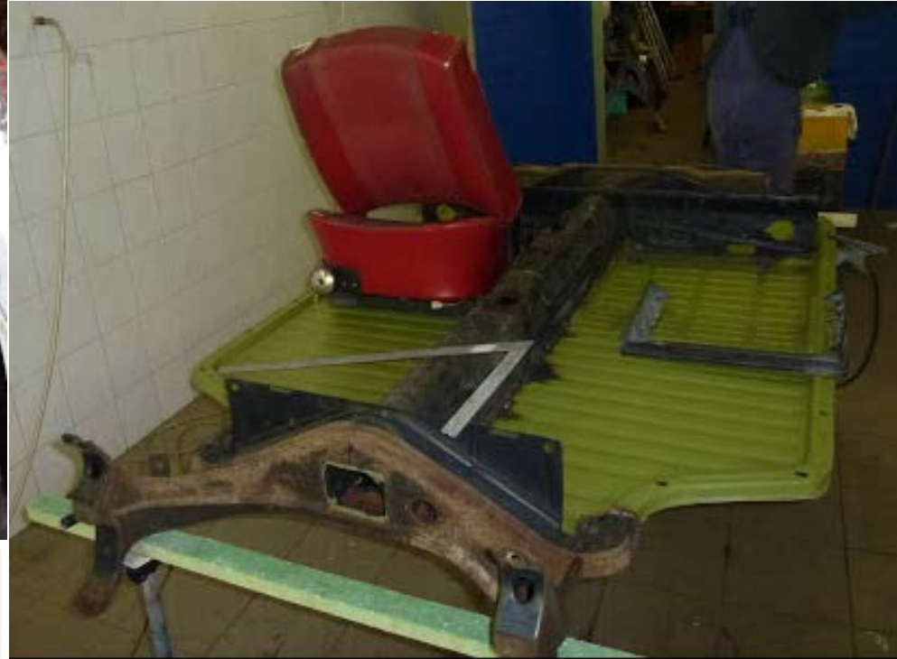
Above: To facilitate the alignment of the body mounting holes with the floorpan holes, Michael had the body mated onto the chassis again.
